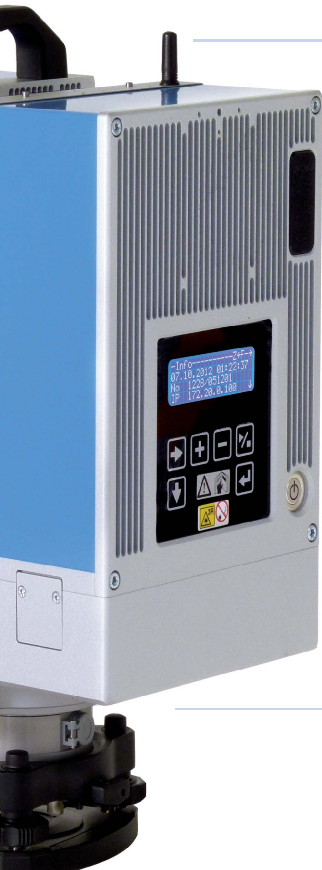
External power supply and Ethernet at the non-rotating scanner base
