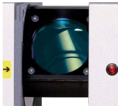
Rotating mirror for 310 vertical scanning
